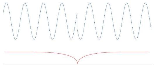
As the 75Hz base frequency, the modulation is generated at central locations, but when the code changes from one code to another (also at the section border), or if the train moves to an area covered by a different "code relay", the phase can change with any value (figure 5).
