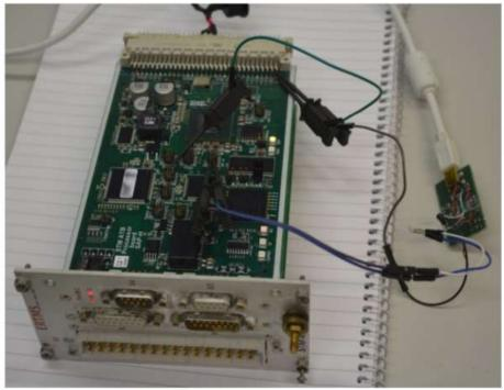
Figure 30: Hardware connections for loading the software on the netX processor [Figure 2250A <<vervangen>>]
