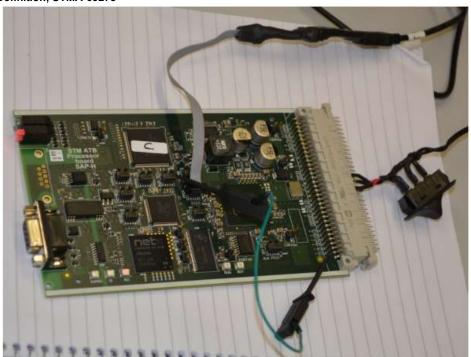
Figure 47: Hardware connections for loading the software on the FPGA processor [Figure 2235A <<veryangen>>]
