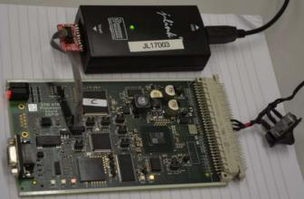
Figure 17: Hardware connections for loading the software on the TIVA co(processor) [Figure 2223A – 2226A <<veryangen>>]
